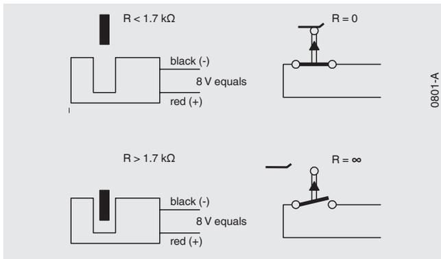
The control unit works, practically, without any reaction on the measuring system. The non-contact "contact system" produces no wear within the electrical system. The installed dimensions correspond to those of the model 821 contacts. The setting of the setpoints is made in the same way as for those contacts.
